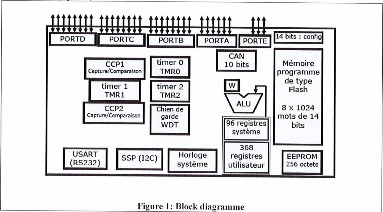
Figure 1: Block diagramme
