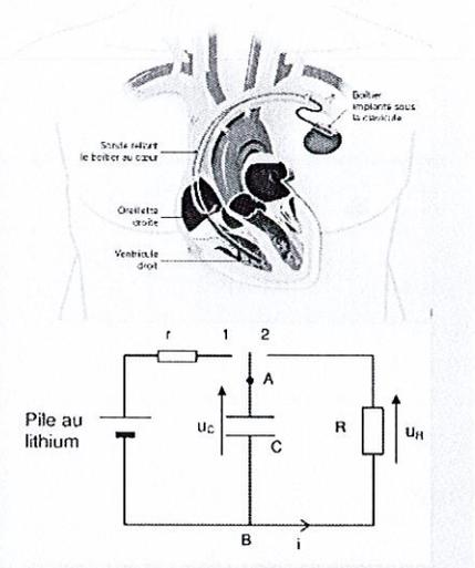
**Données :**  $E = 5,6$  V ;  $C = 0,40 \mu\text{F} = 4,0 \cdot 10^{-7}$  F ;  $r = 1,0 \text{ k}\Omega = 1,0 \cdot 10^3 \Omega$  ;  $R = 2,0 \text{ M}\Omega = 2,0 \cdot 10^6 \Omega$
